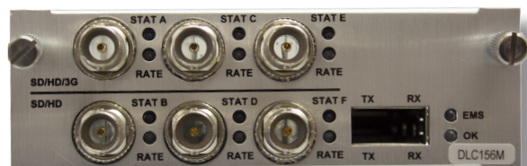
DLC156M rear panel video I/O, XFP cage and status LEDs
